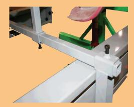
The 4 center uprights bolt directly to the body mounts in the center of the Corvette on the birdcage.
